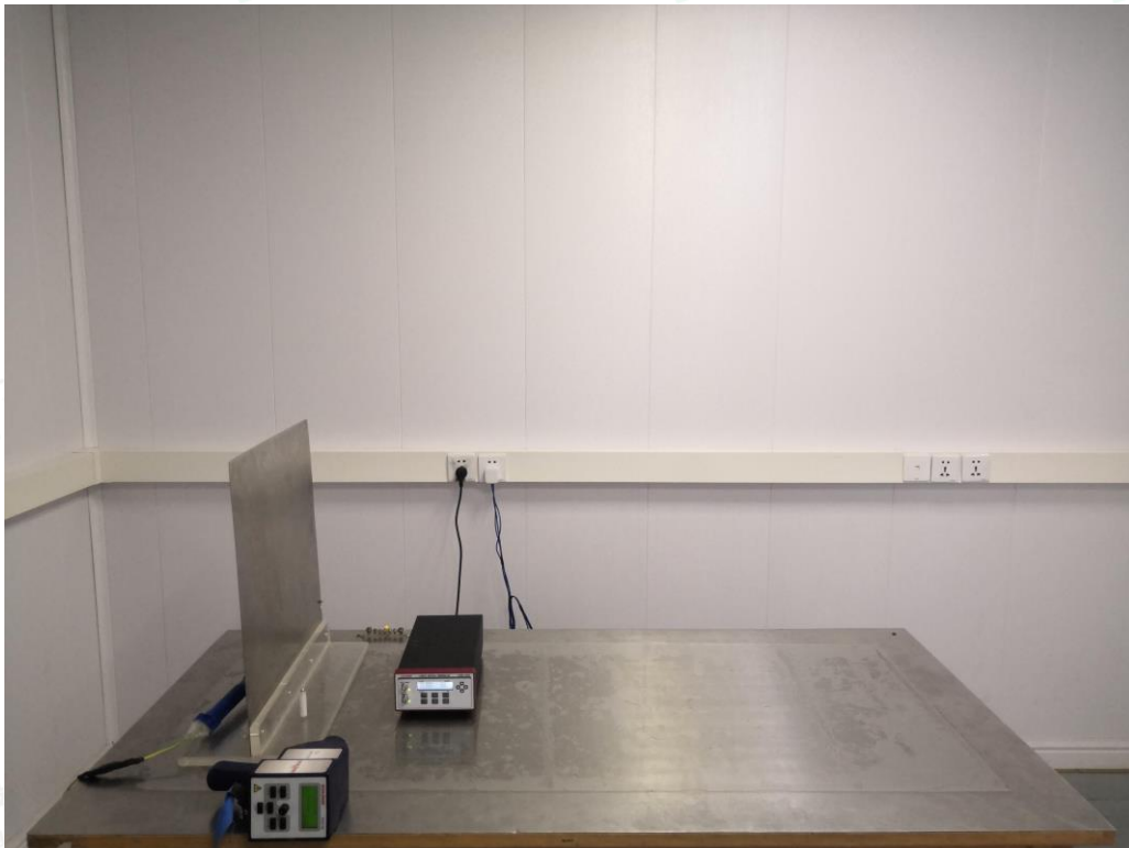
Test Setup Photo of Electrostatic Discharge Test
