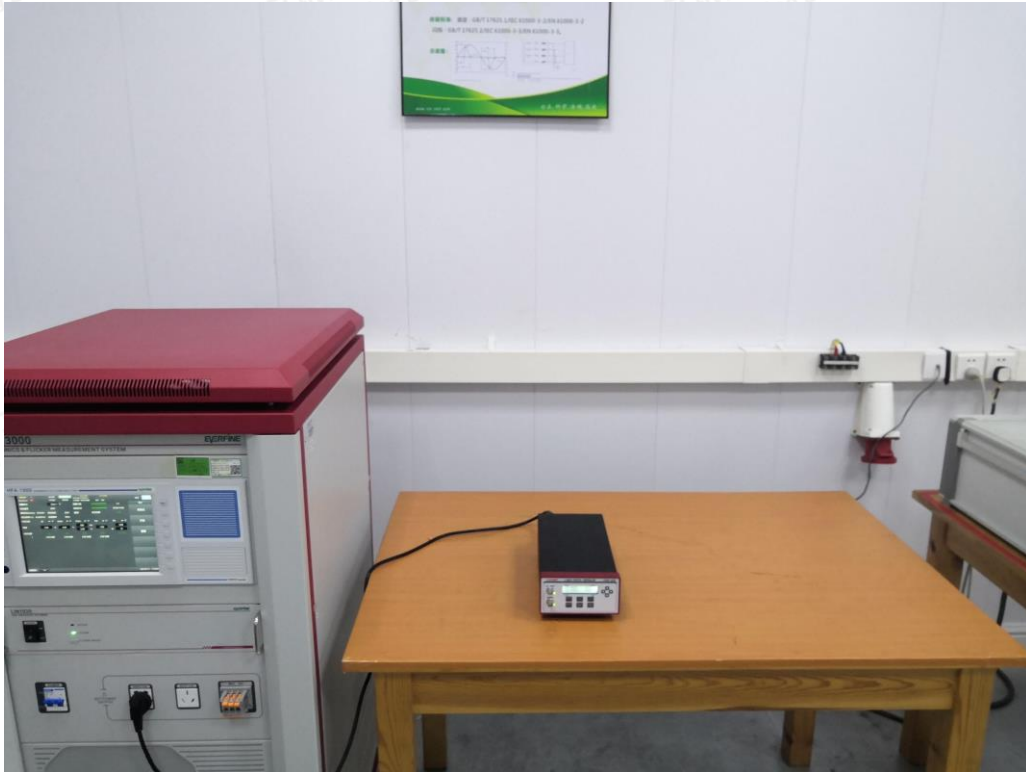
Test Setup Photo of Harmonic & Flicker Measurement
