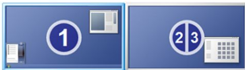
Figure 129: SLM display configuration to be used as an extended screen with a mirrored additional monitor. “1” is the primary monitor, “2” and “3” are the SLM and the additional monitor. A decent graphics card might be required for this setup.
