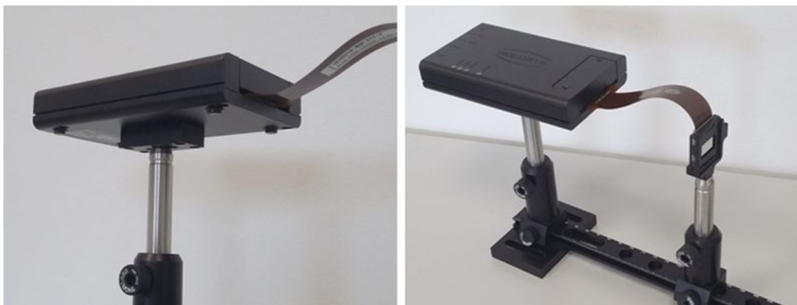
Figure 15: Left image : Device mount attached to device driver. Right image : Complete setup with device mount and display mount on posts.
